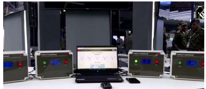
'Vidyut Rakshak': Indian Army officer's innovation to operate multiple generators from single system remotely
